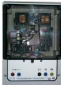
ST 05 DC / AC inverter / mains parallel operation
